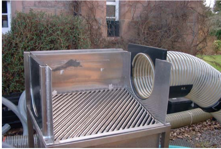
Figure 1 – The Dewatering tank setup for right-handed entry.
